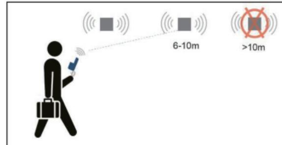
The range for which a smart phone can communicate with the product is dependent on the smart phone Bluetooth capability. The position of the product and the environment between the smart phone and the product can also affect the communication.
