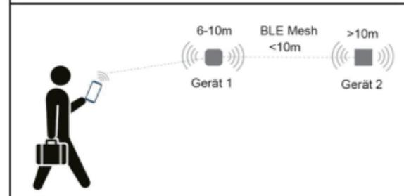
With BLE Mesh, the distance between the smart phone and the product can be more than 10m.
